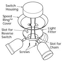
Figure 7d - Attaching Light Fixture
